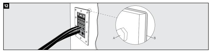
Make sure that bolted frame types are sealed to the structure. All attachment points (A) shall be used and the gasket (B) shall be visible.
