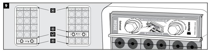
Verify that the stayplates have correct positions and that the wedge has correct orientation.
