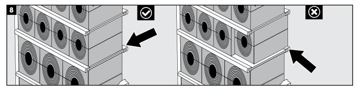
Check that all modules are installed between the edges of the stayplates.
