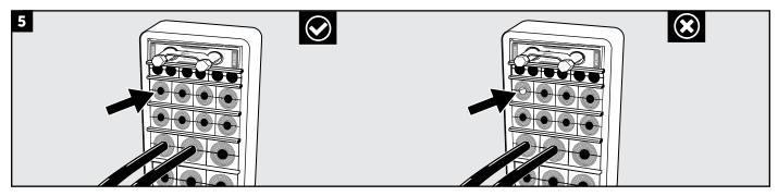
Check that no center cores are missing.
