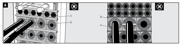
A = Too many layers removed. B = Not enough layers removed. Check that there are no visible gaps between cables/pipes and module halves after compression. Maximum one layer difference is allowed between module halves within the same module.
