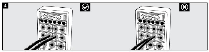
Check that only one cable/pipe passes through each module or opening in a module.
