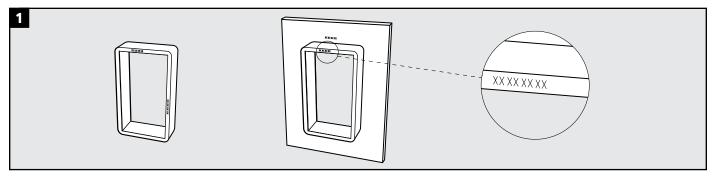
Verify that an original Roxtec frame is used. An original Roxtec frame is identified by a Roxtec marking or a frame serial number marking. Frames have the marking or label on the front face.
