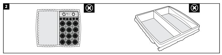
Check that the transit and packing system have no mechanical damages. Also check surface protection and welds if applicable. For welds, see Roxtec welding guidelines.
