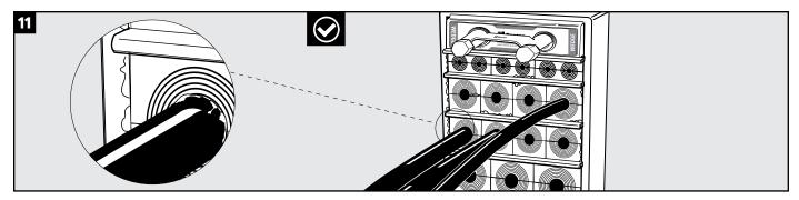
Check that the frame and the modules have been lubricated. Excess lubricant shall be visible directly after installation.
