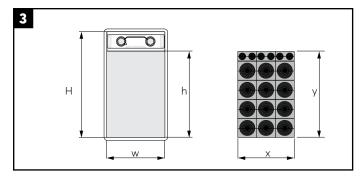
Verify the correct utilization of the entire packing space. The total width (x) and total height (y) of the installed modules shall correspond to the packing width (w) and packing height (h) of the frame.
