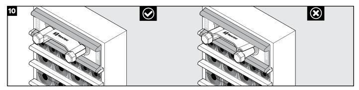
Verify that the wedge is fully tightened.
